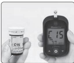
2. It recognizes automatically the code number. This is a very convenient function preventing the inconvenience of setting the code number on the blood glucose test meter every time.
