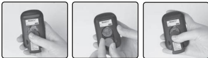
Your Glucofine® blood glucose test meter uses only two 3V Lithium batteries (CR2032), which are included. When replacing the batteries, only CR2032 or equivalent lithium battery should be used.
